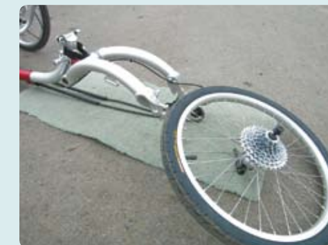
3 Now remove the rear wheel. Like any derailleur bike, it's easier if you change to the smallest ring and cog first.
