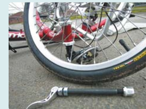
6 Undo the front wheel quick-releases, and unscrew the lock nuts from behind the kingpins. The axles can then slide out, freeing the wheel and also releasing the drum brakes. Take care that the spacer doesn't go astray.
