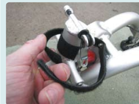
4 This Velcro strap prevents the rear swingarm flopping under – release it now.
