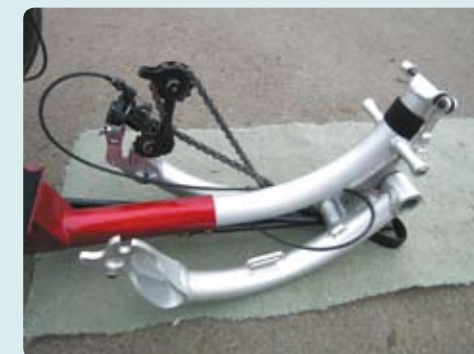
5 That lets you fold the rear swingarm under. You need to hold the chain tubes up as you do this so the chain doesn't get caught up.
