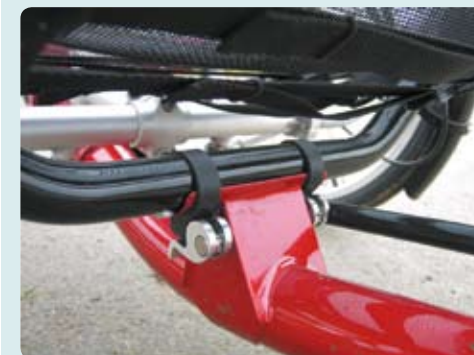
1 First, undo the two quick-releases on the plastic seat clamps and wiggle them off.
