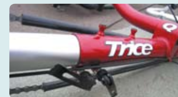
8 At this point, stop and see if it's small enough yet! If you do need it smaller, undo the QRs and withdraw the front boom until it comes out. There's a plastic sleeve so it slides reasonably easily in the frame, but pulling it right out and avoiding scratching the frame on the ground as you do so is a bit awkward. It also loses your leg-length adjustment, so it's best avoided if you can. You may also need to unhook the front derailleur cable and swing the left-hand handlebar forward to create enough slack.
