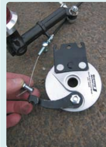
its wheel and push the QR axle through, and thread on the spacer and lock nut, so it's all held neatly together.
