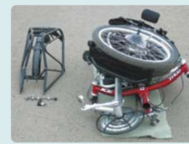
10 Pile all the bits up and it goes impressively small. With a bit more effort no doubt I could have slotted the rear rack into the pile, too. If you're going to pile it up like this, you may as well leave the handlebars in their upright, riding position to keep it all together.
