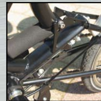
The Bike Friday Tikit rear swingarm uses the flexibility of the metal plates to hold it in place on the boss (with Allen bolt head visible) on the main frame. Below you can see the anchors for the stem release cables, and to the left is the foam-covered handle for ‘trolley mode’.
