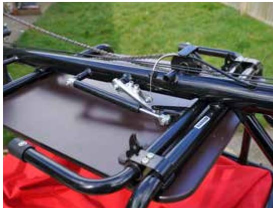
**ABOVE: Underside view of the cable-operated stand release.**
