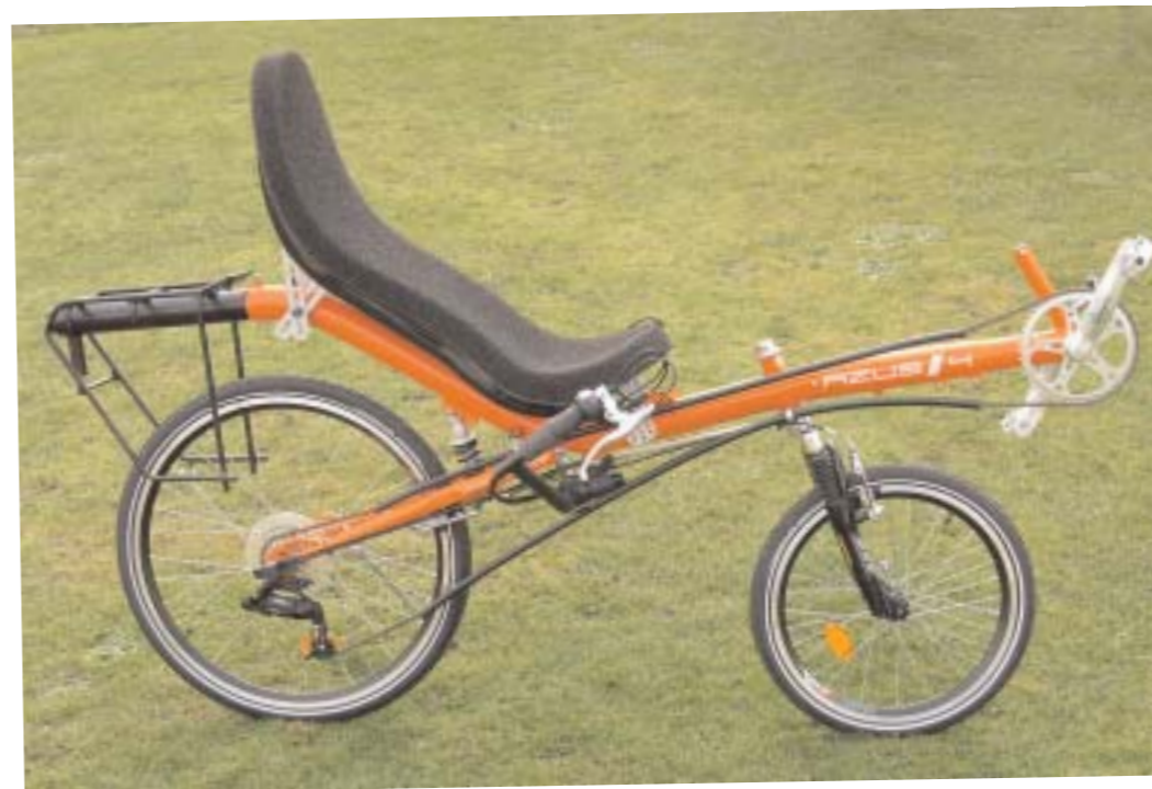
BOTTOM ROW: The DualDrive controls are operated between thumb and forefinger as intended, with some neatly managed, if tight-radius, cable runs. The carrier rack is super-solid, if a bit far back. Mudguards are an optional extra, incidentally, and eyelets are in place on the frame to accept them. And, shown below, there's a choice of suspension setting via a row of mounting holes for the shock.
