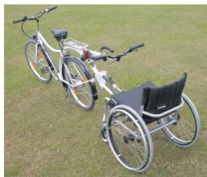
RIGHT: The 'Speedy' tandem imported by Bromakin Wheelchairs enables the wheelchair user to attach and detach unaided.
