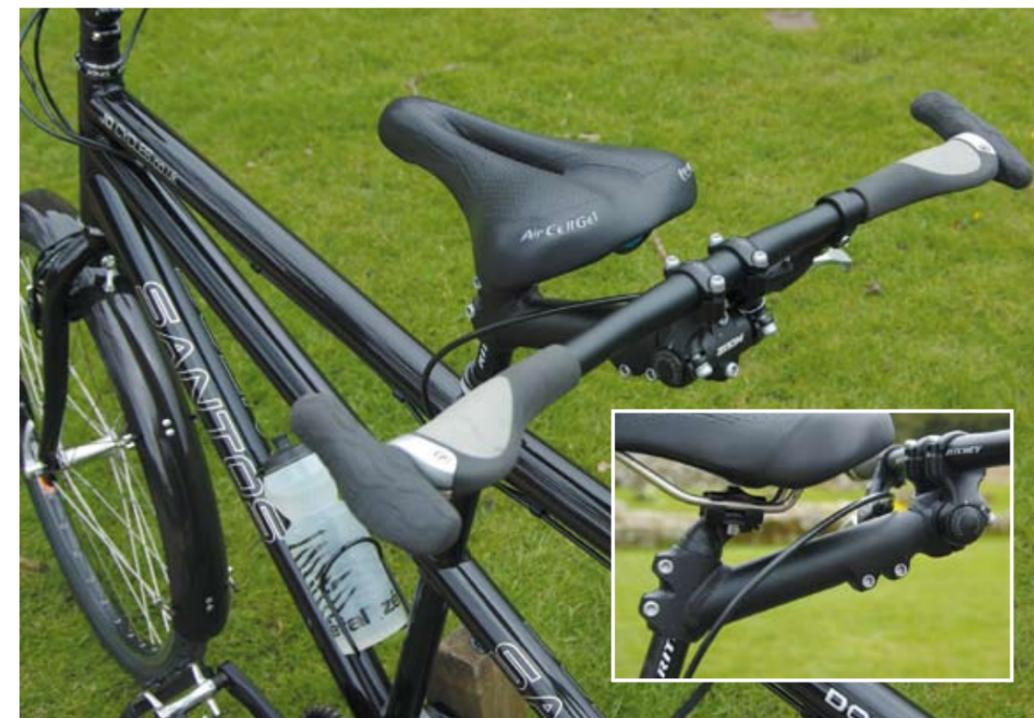
**ABOVE:** The handlebar setup is the same for both riders: Ergon grips and Ergo bar ends. The stoker stem is solid and adjusts for length.
