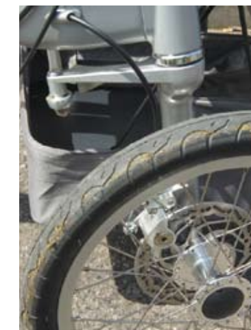
ABOVE: Disk brakes on the front wheels provide good stopping in the 16" (305) wheels.
