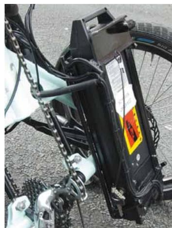
**ABOVE:** Access to the battery is easier if you tip the trike up. Note the captive key (in the battery lock/switch) on its steel tether.
