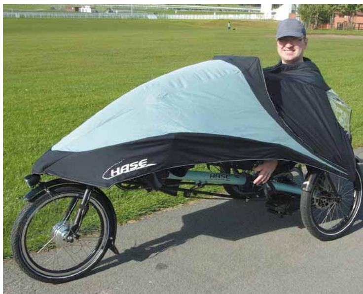
the steering loved to flop right round to one side – perhaps a steering stabiliser spring would be an idea. Also, I found it very tricky to lift or carry the machine with the fairing up, so in wet weather this ruled out a number of my possible routes to work where steps or barriers were involved. Similarly, you really do need a garage or large shed to store it in; it stands neatly on its end but still takes a bit of space to wheel in and lift up.
