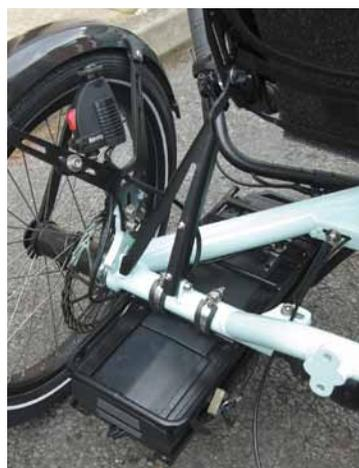
**ABOVE:** The battery is housed in a metal frame down near the left rear wheel. With the weight so low there's little effect on the handling.
