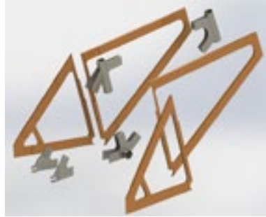
ABOVE: Main frame comprises five steel assemblies and four plywood sheets. The fork is, as yet, steel.
