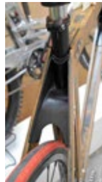
ABOVE: Main frame comprises five steel assemblies and four plywood sheets. The fork is, as yet, steel.
