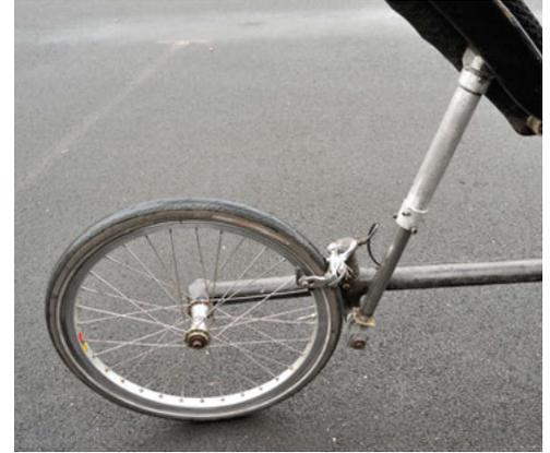
**ABOVE:** Mark made his own gas strut to assist the transition between ride heights. The cantilever rear axle is, he says, the simplest mounting option for a single-spar frame.
