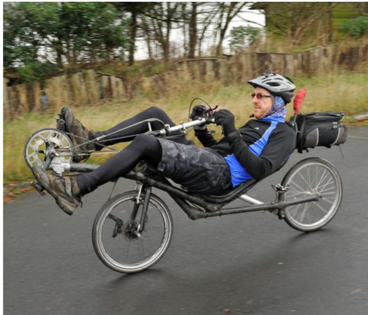
**ABOVE:** Low-ride position is deployed by a 'winching' mechanism when back-pedalling.
